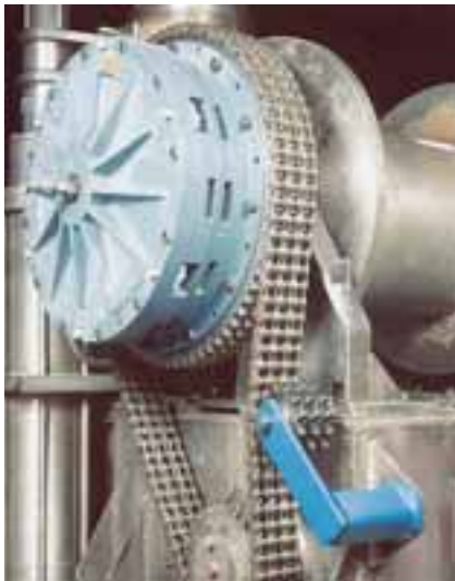
Chain tensioner on drilling machine in mining industry
