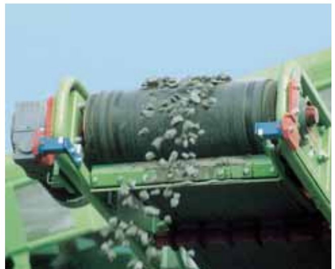
Elastic suspension on belt scraper
