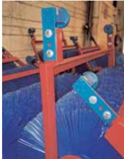
Suspension of circular brush on potato harvester
