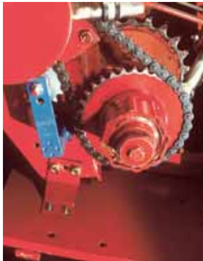
Chain tensioner on baling press
