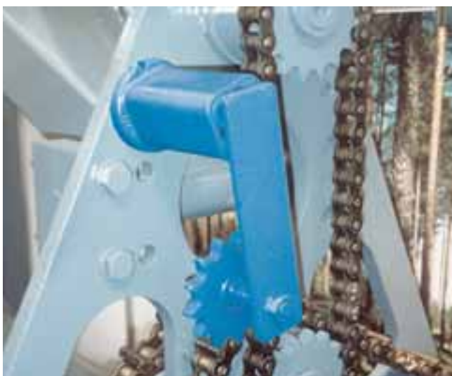
Chain tensioner on paper rolling mechanism
