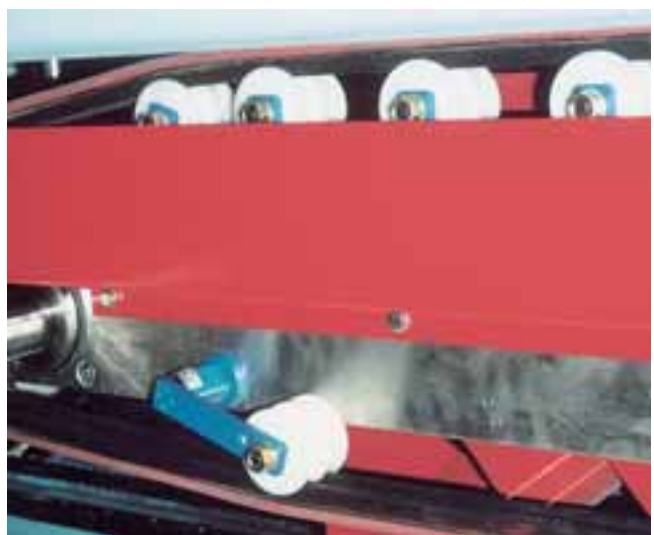
Belt tensioner on material intake in a grinding machine
