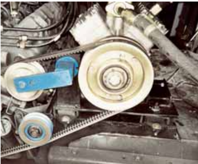
Belt tensioner on belt drive for an AC-compressor
