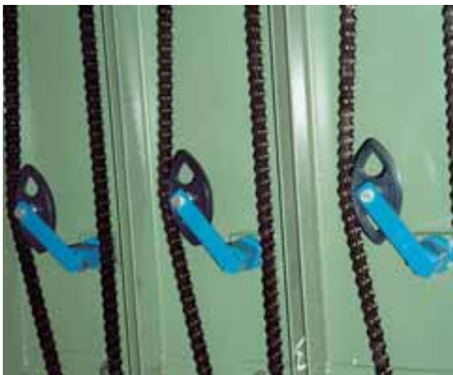
Chain tensioner with glider on processing machine
