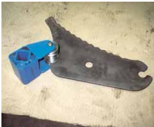
Elastic suspension of shaping knife in baler
