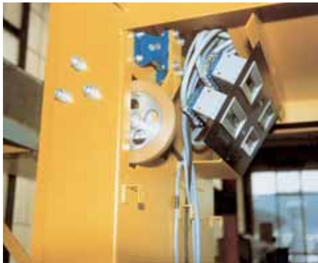
Elastic suspension of caliper roll in elevator
