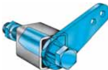
Fig. 14 Lever connection with one through bolt
