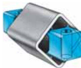
Fig. 16 Inner square section made of solid metal and cross bores on both protruding sides
