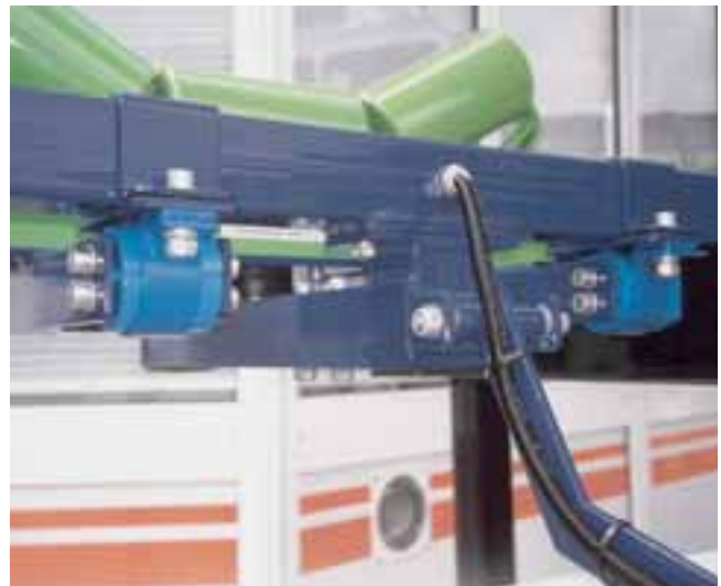
"Floating" suspension of weighing device in belt conveyor
