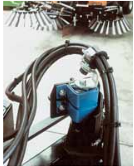
Suspension of a brush in road sweeper
