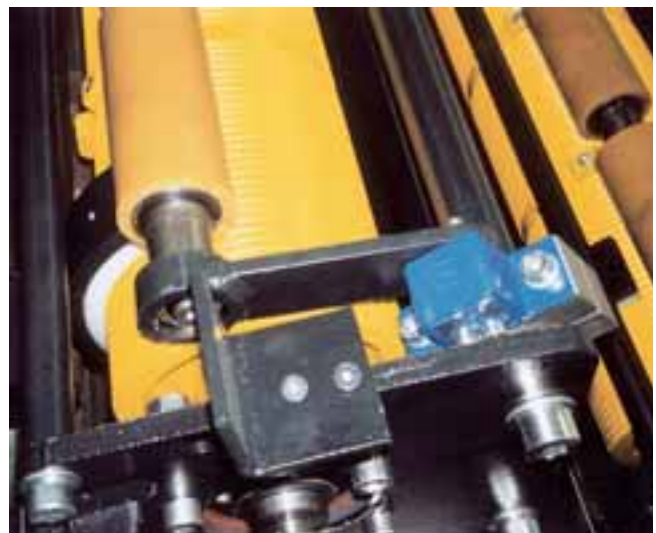
Elastic caliper roll suspension in cardboard rolling machine
