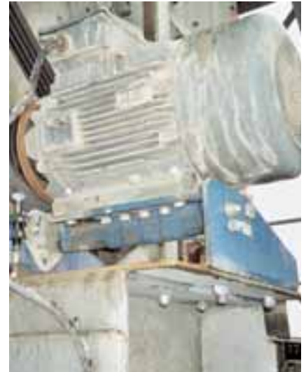
MB motor mount on dewatering screen
