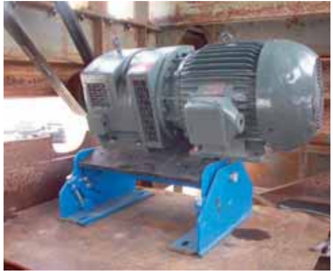
MB 70 with variable speed drive for crusher
