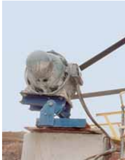
MB 70 motor mount in crusher
