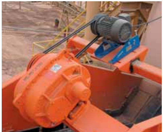
MB 50 with drive motor for exciter
