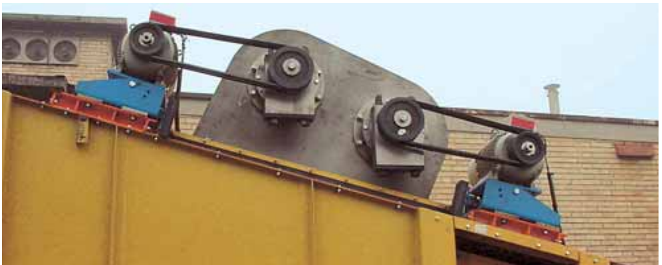
MB mounts of drives on asphalt screen
