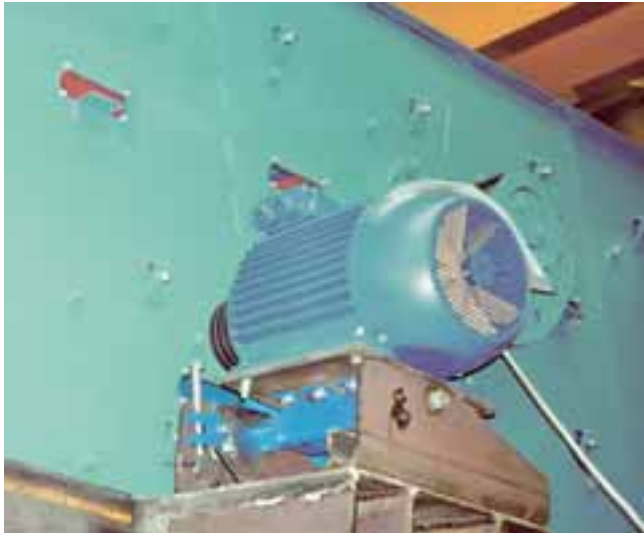
MB 50 for belt drive on circular motion screen
