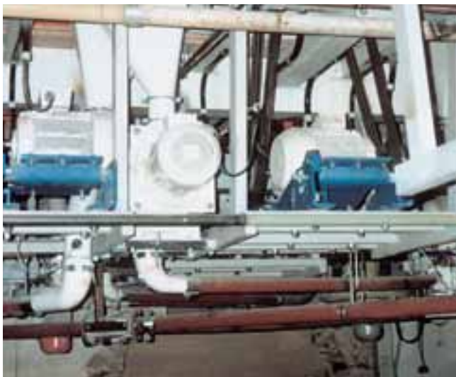
MB 50 with drives for roller mills
