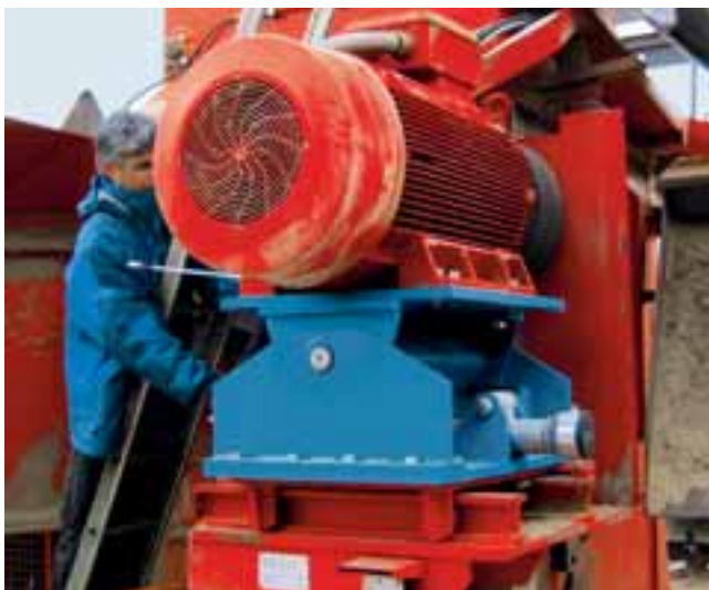
Elastic suspension of chipper-drive with MB 100
